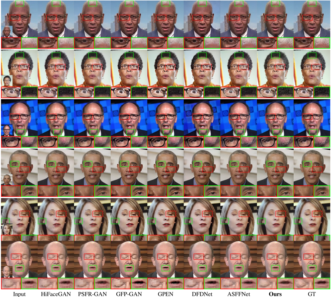
Figure 7. Qualitative comparison between the proposed approach and the baselines for the HDTF dataset and CRF 42. The bottom-left image in the input column represents the reference frame exploited by our approach. Best viewed in full screen.
